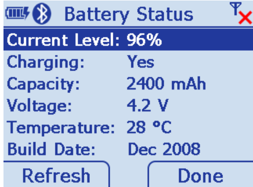
Figure 2-9 Battery Status Screen
